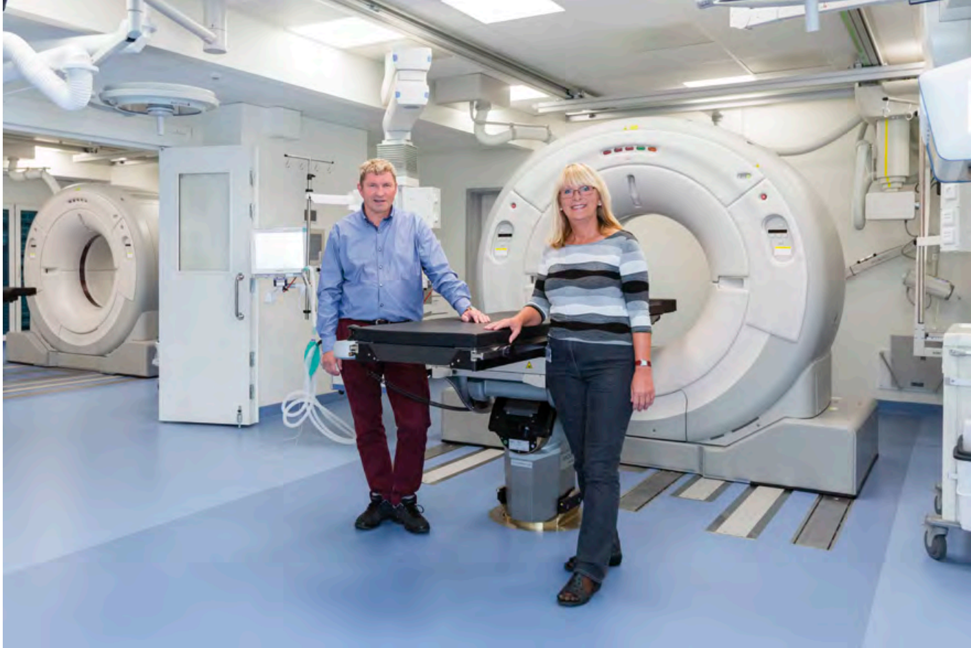
Ilse Vejborg and Johnny Madelung in front of one of the two Aquilion LB 32-slice Sliding Gantry CT scanners at the World Class Trauma Center at Rigshospitalet.
